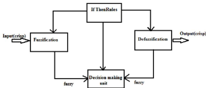
Fig. 2. Block diagram of fuzzy logic.
