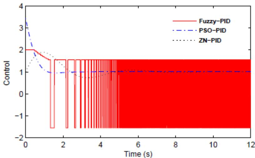
Fig. 6. Control efforts of system for fuzzy, PSO-PID and PID controller.
