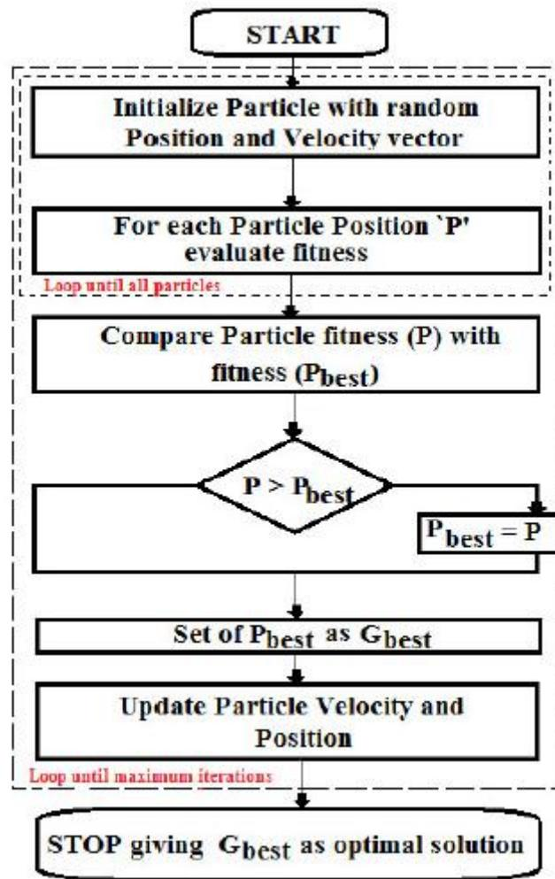
Fig. 4. Flow chart on evaluation of PSO algorithm [12].
