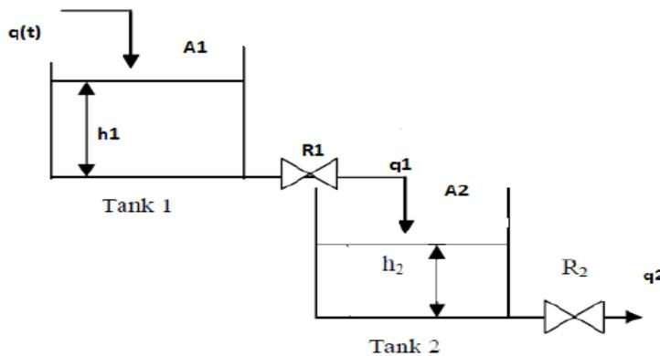
**Fig. 1.** Two Tank non-interacting process [21].
