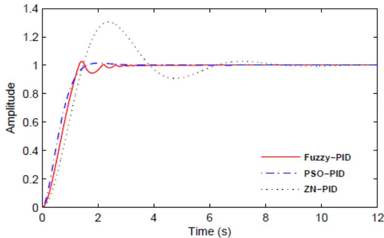
Fig. 5. Response of system for fuzzy, PSO-PID and PID controllers.
