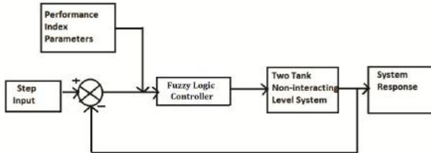
Fig. 3. Fuzzy controller for two tank non-interacting system.
